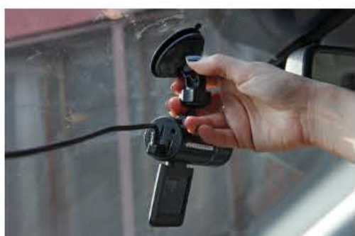
STEP 1: Mount Dash Camera on windshield behind rear view mirror.
