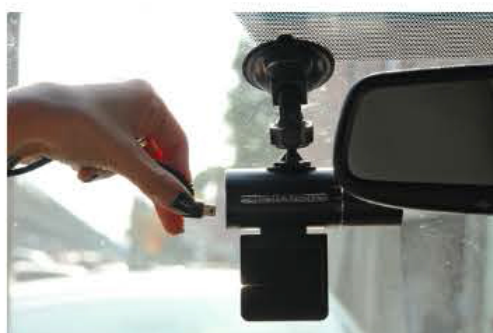
STEP 3: Attach power cable to the dash camera.
