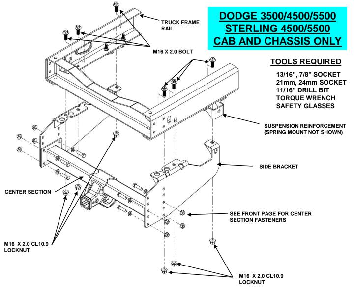
General assembly - loosely install side brackets on vehicle (this page); install center section assembly and tighten all fasteners to proper specifications (page 1)
