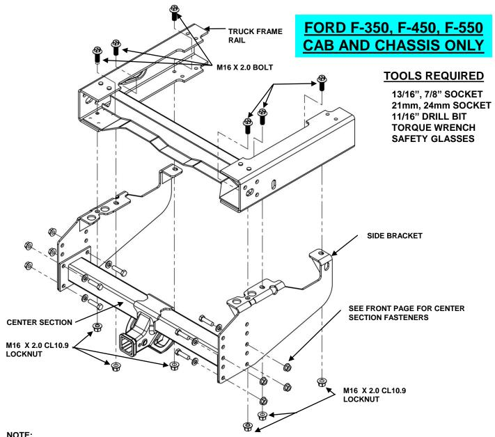
General assembly - loosely install side brackets on vehicle (this page); install center section assembly and tighten all fasteners to proper specifications (page 1)
