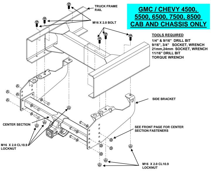
General assembly - loosely install side brackets on vehicle (this page); install center section assembly and tighten all fasteners to proper specifications (page 1)
