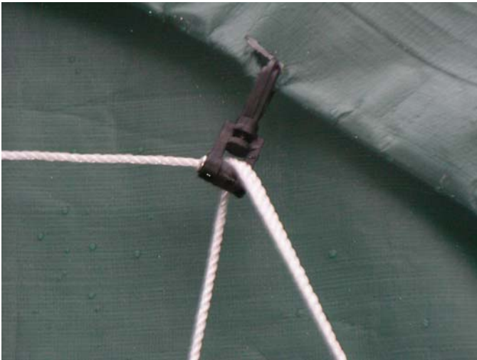
Roller installs on outside rope channel of door
