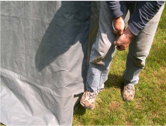
Remove Slack From Cover Rope
