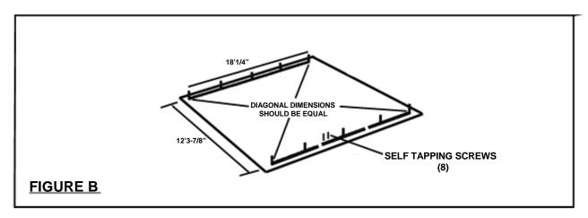
4. After you have completed all measurements and have the End Base (5) and Center Base (6) Rails in place and squared, screw the joints together with two Self Tapping Screws (8) per joint on the top surface of the Base Rails. (See Figure B.)
