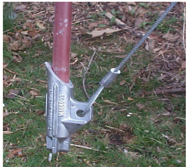
Drive Rod inserts into Anchor Head
