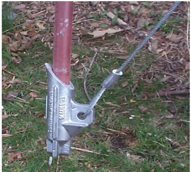
Drive Rod inserts into Anchor Head
