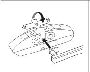
Attaching the **"D" adapter**: Place adapter over the metal anchor on the back of the wiper blade; slide the adapter into place. Once it is in the proper position you will hear a click. Try sliding it forward gently. If it doesn't move it is installed correctly.
