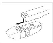
Attaching the **"B4" adapter**: Line up the round holes of the adapter to the round anchors of the "B" base. Push the adapter down until it clicks onto the "B" base.
