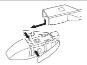
Attaching the wiper blade to 19mm wiper arms: On the **"B2"** adapter there are two wing anchors on the back end of the adapter, rotate the wing anchors so they are facing the back of the adapter as pictured. Slide the adapter into the wiper arm until you hear a click. Pull on the blade to make sure it is properly fastened.
