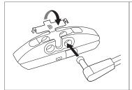
Connecting the arm to the blade: Remove the retainer in the center of the "D" adapter by squeezing the clips on either side of the adapter and pulling up. Slide the side pin of the wiper arm into the hole on the side of the adapter (1/4" larger hole and 3/16" smaller hole), then reinstall the retainer on the top of the adapter. Pull on the blade to make sure it is properly fastened.
