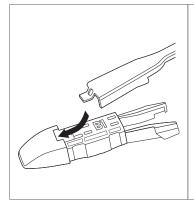
Attaching the "B1" adapter: Line up the round holes of the adapter to the round anchors of the "B" base. Push the adapter down until it clicks onto the "B" base.
