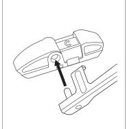
Attaching the **"C" adapter**: Place adapter over the metal anchor on the back of the wiper blade; slide the adapter into place. Once it is in the proper position you will hear a click. Pull on the blade to make sure it is properly fastened.
