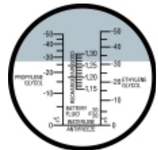
The reticle with liquid on the prism. The reading is taken at the point the shadow line crosses the scale.
