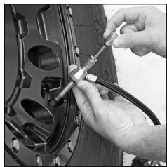
5) Push the valve core remover down, turn it until you feel it lock onto the valve stem and then unscrew the valve stem until it comes completely out into the deflator unit.
