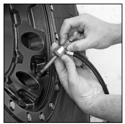
**4)** After removing your valve stem cap, hold the sliding valve tight and thread the unit onto your valve stem threads using the knurl on the valve stem adapter.
