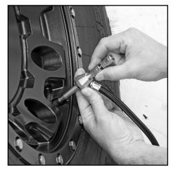
10) Hold the sliding valve and unscrew the valve 11) Replace your valve stem cap. stem adapter from your valve stem.
