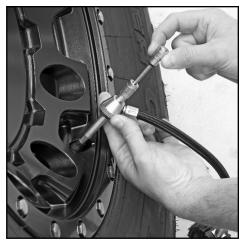
9) Once you have reached your desired tire pressure, screw your valve stem back in using the valve core remover.
