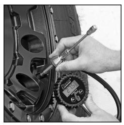
**6)** With the valve stem out, you can now push the sliding valve down until it stops to read current tire pressure. This tire is currently at 27.5 pounds of pressure.
