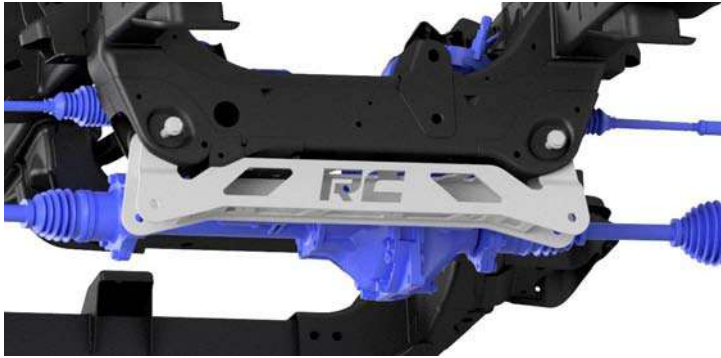
Install front crossmember.
