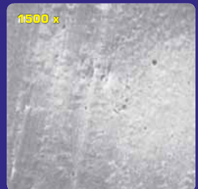
The bearing is visibly smoother after using Royal Purple HPS.
