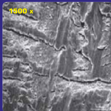
The bearing is scuffed after using a leading synthetic motor oil.
