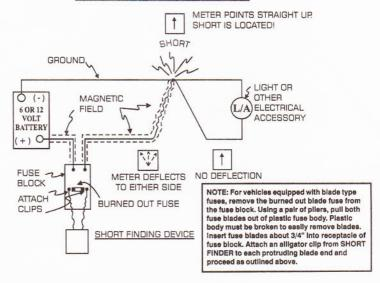
NOTE: BEFORE USING THIS DEVICE, CONSULT THE VEHICLE SERVICE MANUAL FOR SPECIFIC CIRCUIT DIAGRAMS IN EACH FUSED CIRCUIT AND ANY PARTICULAR TEST OR REPAIR PROCEDURES. NOT RECOMMENDED FOR TESTING ELECTRONIC ENGINE OR BODY CIRCUITS INCLUDING: COMPUTERS, SENSORS, FUEL INJECTORS AND AIR BAGS.
