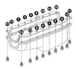
**Step 5** - Torque oil pan bolts. Basic torque specifications for Chrysler, Ford, and GM engines.
