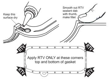
**Step 4** - Install SCE "One-Piece" oil pan gasket to engine block paying close attention to tab inserts at rear main cap and front cover assembly, then set oil pan in place carefully. Install oil pan bolts and torque to manufacturer's requirements in sequence, "crush limiters" will prevent damage to gasket from over tightening.
