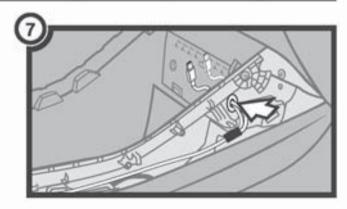
8. Run the remaining type-c connection along the support frame and the trim panel leading to the 12v socket exposed in step 4 of the disassembly.
