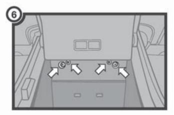
1. Removing the phone placement panel may require a bit of force when pulling the panel away.
