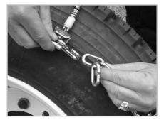
Connect the "speed hook" on the inside of the tire (the side away from you). As a starting point, we recommend that you fasten it so that there are no more than two "free" links. It may be necessary to drive forward two to three feet so that the inside connection can be made more easily.
