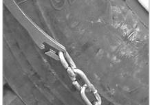
Connect the outside fastener at it's loosest setting, then pull the cable towards you to create as much slack as possible. Make sure that none of the cross members are caught in the "shoulder" area of the tire tread.
