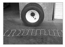
Park vehicle on firm level ground, away from traffic. Unroll the set and lay each half pair on the ground next to the tire it is intended to cover. Make sure that there are no twists or kinks in the cable chain.
