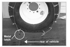
Drape the chain over the top of the tire so both ends can touch the ground and the long metal latch is on the outside of the tire (toward you) and is draped toward the back of the vehicle. The two half sets are made so that one fits only on the left and one only on the right. See Close-up below
