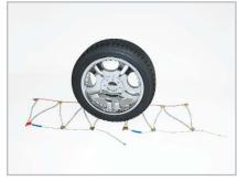
Move the chain is a sweeping motion under the vehicle so the open midsection is positioned up against the backside of the tire. This sweeping motion can best be done while kneeling in front of the tire.
