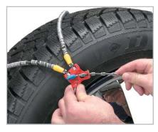
Grasp the outside cable with both hands and pull it toward you to create as much slack as possible. Connect the top fastener (the red one) as tightly as possible by inserting the silver "beads" on the cable through the keyhole.
