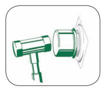
Tap installation tool with mallet until sleeve is seated on shaft over the marked area. Remove installation tool.\*
