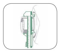
Clean and measure the diameter of the worn shaft and mark the area where the sleeve will cover the scored portion of the shaft.
