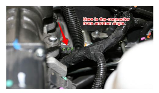
The connector is typically located between the ECM, and the intake horn. On some trucks it may be towards the upper right portion of the ECM. It can vary where this connector is located, but it is usually within a couple of feet from the ECM. Sometimes it is closer to the firewall, and other times it is closer to the front of the truck.
