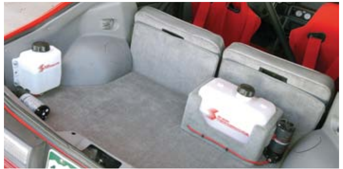
Mounting Example: 3l tank (separate brake cooling) and 9.5l trunk mounting kit with pump
