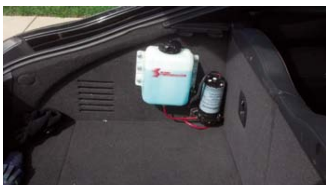
Mounting Example: Audi TTS - 3l Boost Cooler reservoir with pump in the trunk
