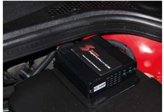
Audi A3 2.0TFSI with Boost Cooler controller within the engine compartment
