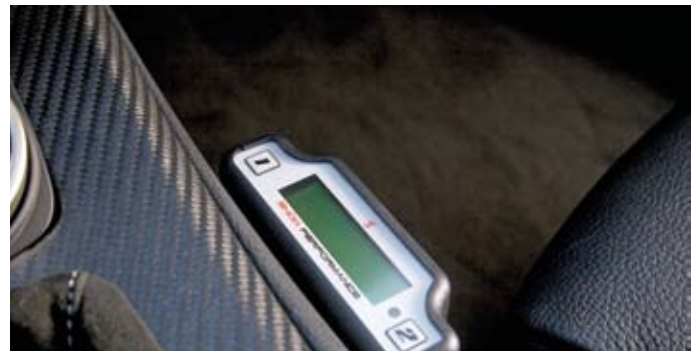
Mounting example: Stage 3 Controller between centre console and passenger seat (BMW E90)
