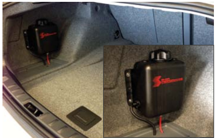
Mounting example: BMW E92 - 3l Tank incl. pump in the trunk (not visible below the reservoir).
