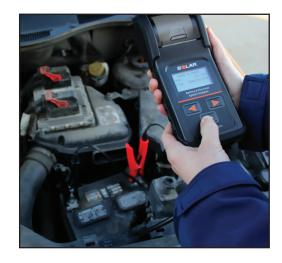
Testing is guick and easy and allows the operator to perform either a battery test, system test or both. The tester walks through the testing sequence, prompting for key pieces of information and guiding the operator from one step to the next. The tester provides accurate assessment of both charged and discharged batteries, saving time and effort.
