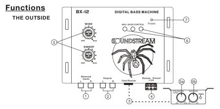
**1. Inputs:** The inputs of TheBX-12 use a balanced input circuit to helpminimize induced noise. The are also designed to handle very high signal voltages up to 15 volts.
