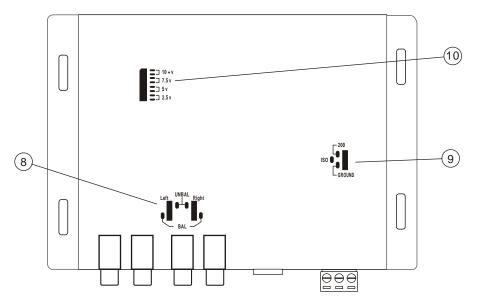
**8. Input Grounding:** For most systems you can leave this jumper set in the BALANCED position. In some systems, the source unit may look for a ground through the RCA connectors. In this event, you should go ahead and change the jumpers to the UNBALANCED position.
