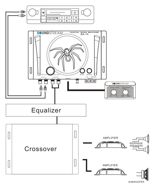
**NOTE:** For signal connection, the output RCA connectors should be connected to the next component after the BX-15, such as a crossover, equalizer, or amplifier. Just remember, the BX-15 should go inline before a crossover.
