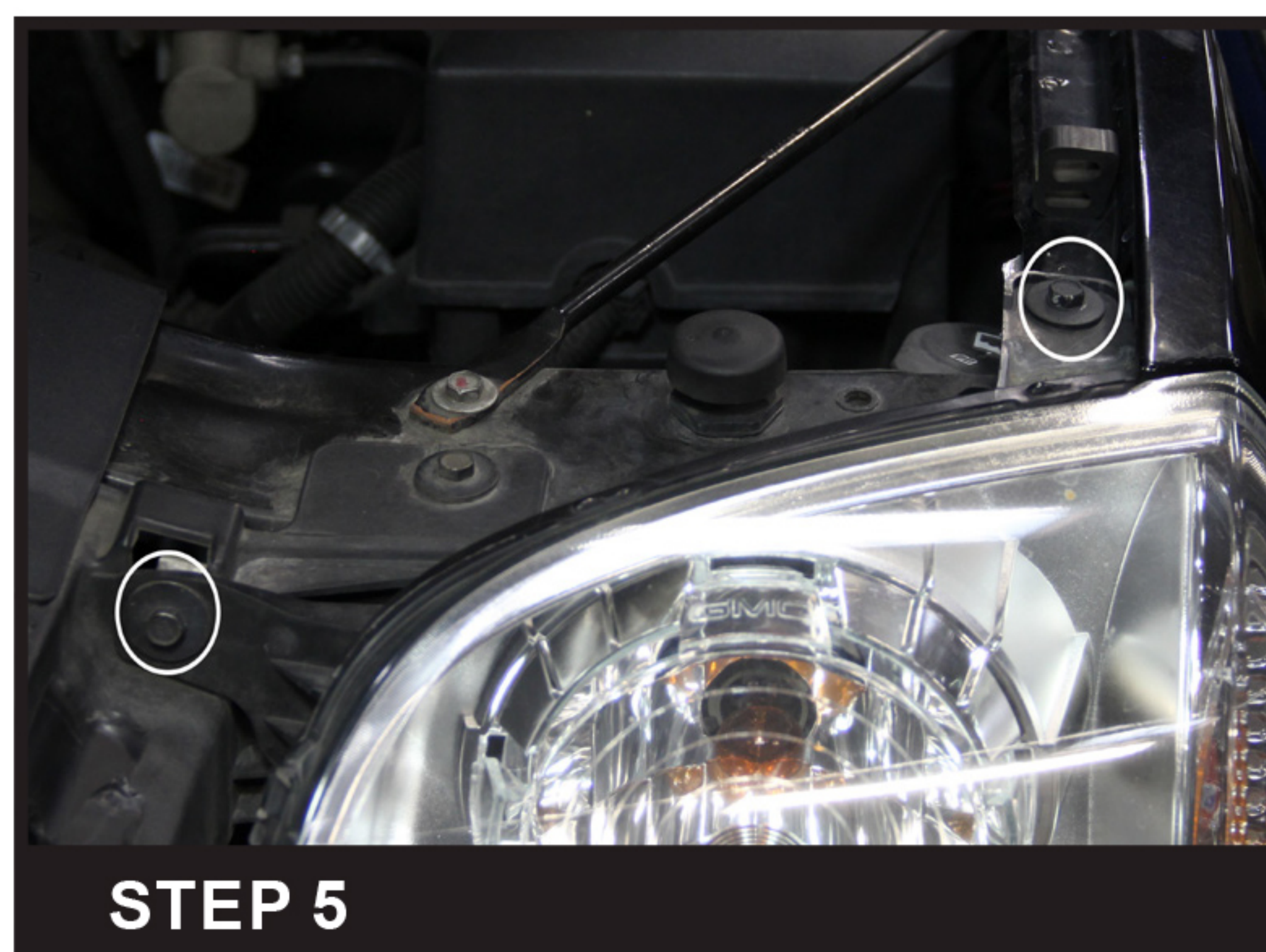
Remove the two 10mm headlight bolts at the top of the headlight
