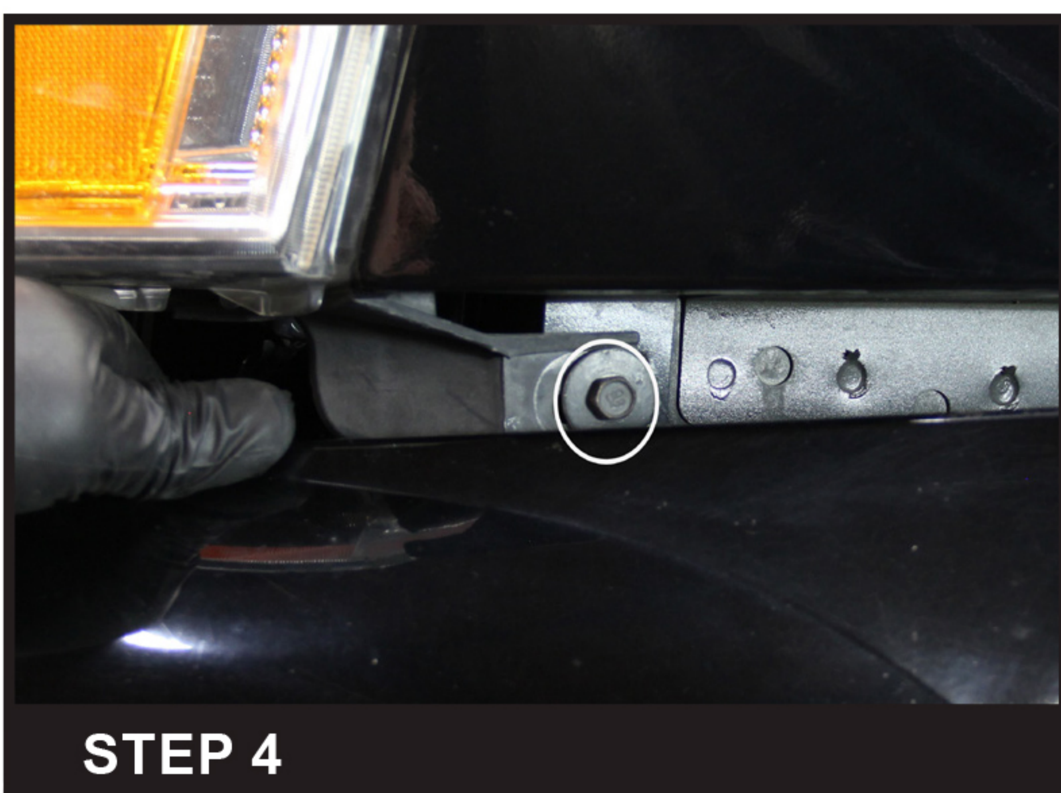
Remove the 10mm headlight bolt at the bottom of the headlight
