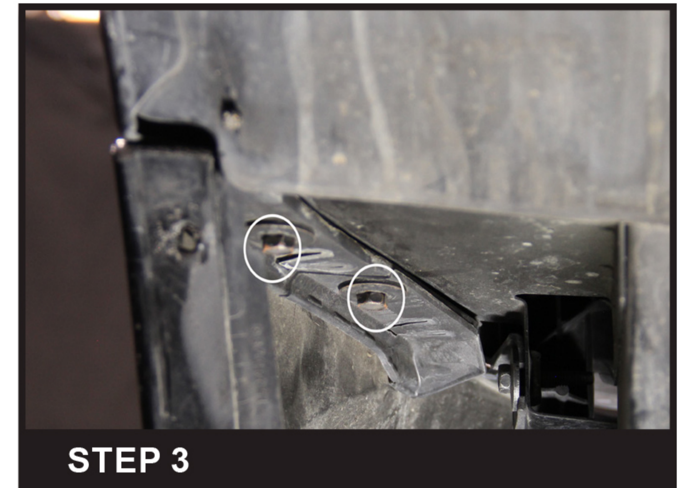
Remove the two 10mm front bumper mounting bolts
