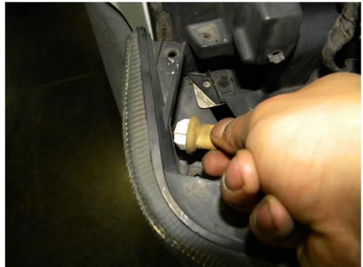
10. Remove the light harnesses and sockets
