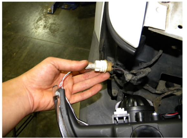
22. Attach the lighting harness to Projector headlight
