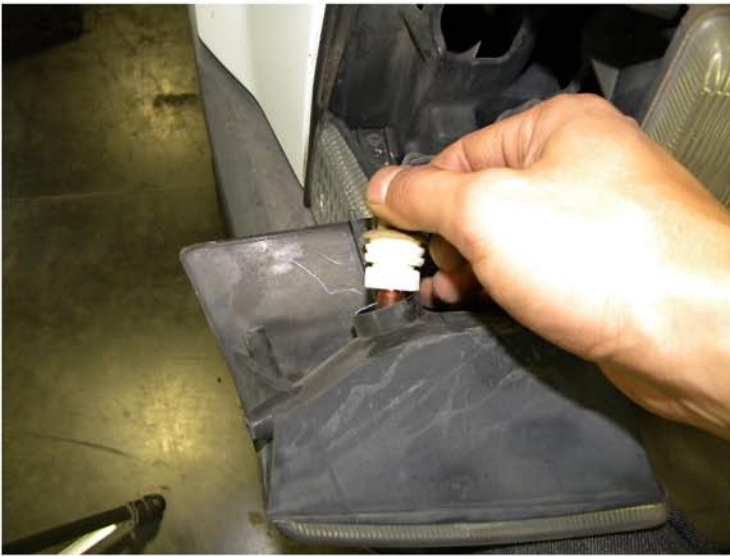
5. Remove the light bulb socket
