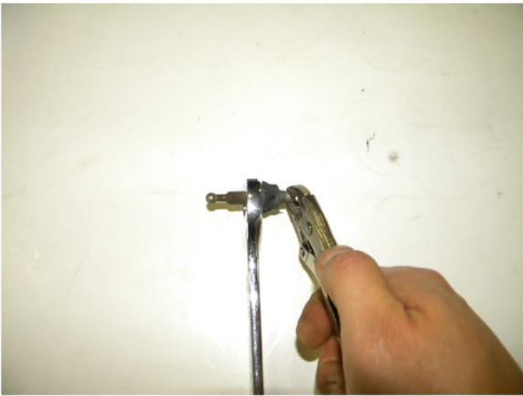
17. Turn the adjustment screw until approximately 4 threads are visible
