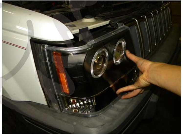
26. Press firmly to attach the projector headlight onto the mounting screws
