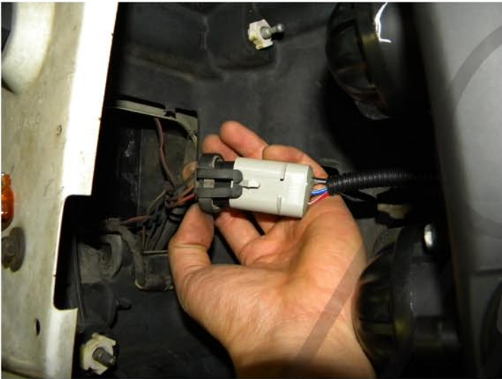
25. Attach the lighting harness to the projector headlight
