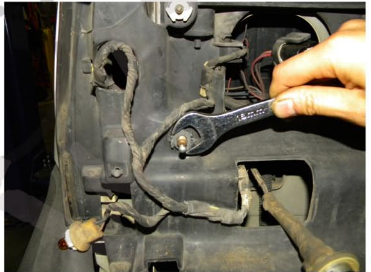
20. Turn counter clockwise to reattach the adjustment screw
