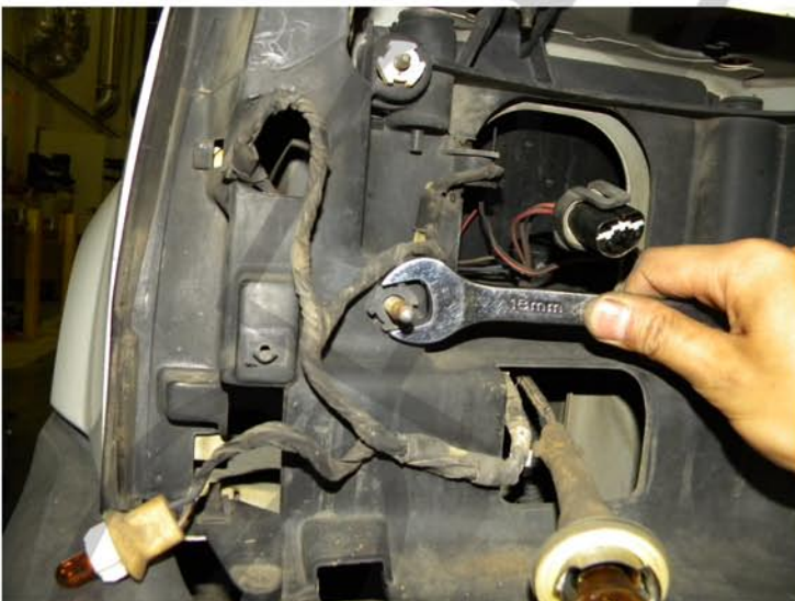
15. Turn clockwise to detach the adjustment screw
