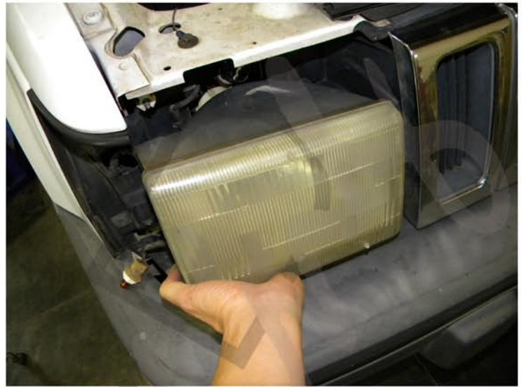
12. Firmly tug on the headlight to remove
