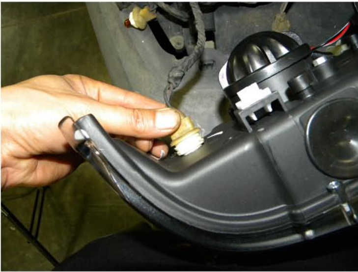
23. Attach the lighting harness to the projector headlight
