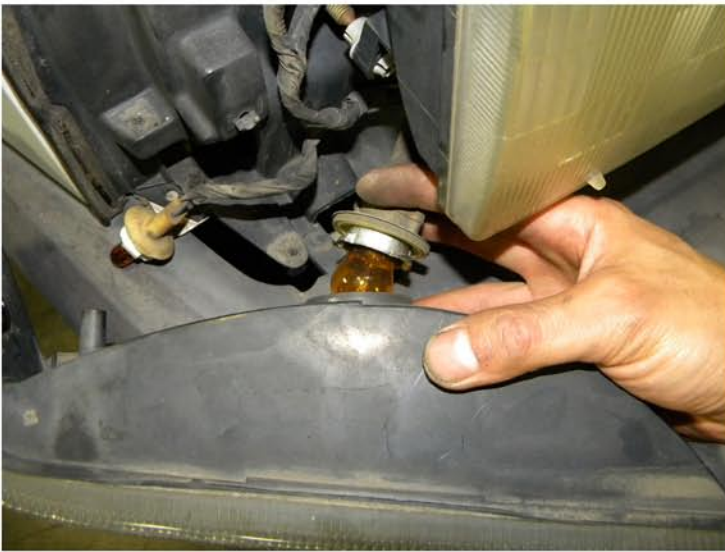
11. Remove the light harnesses and sockets
