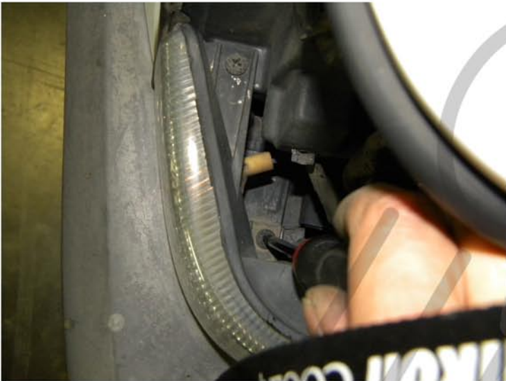
7. Remove the (2) phillips head screws
