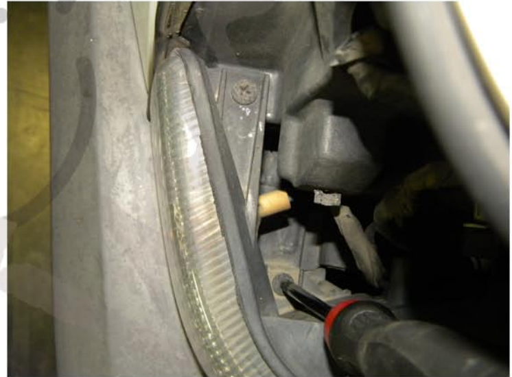
8. Remove the (2) phillips head screws
