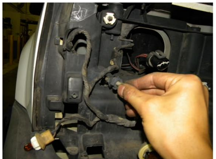
16. Remove the adjustment screw
