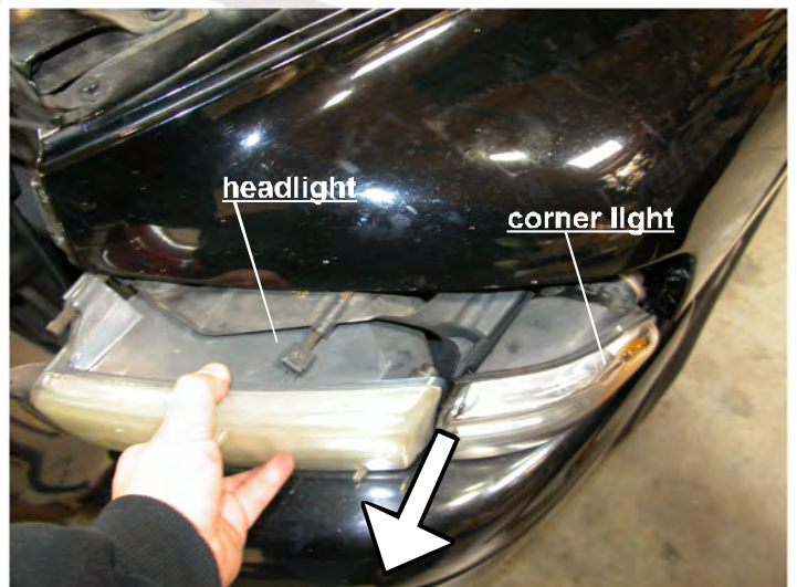
4. Pull out the headlight a little bit first (BOTH SIDE)
