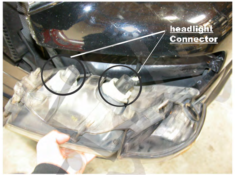
6. Disconnect the connector from headlight (BOTH SIDE)
