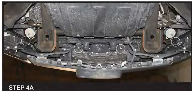
Remove the four 10mm lower grille mounting bolts behind the front grille
