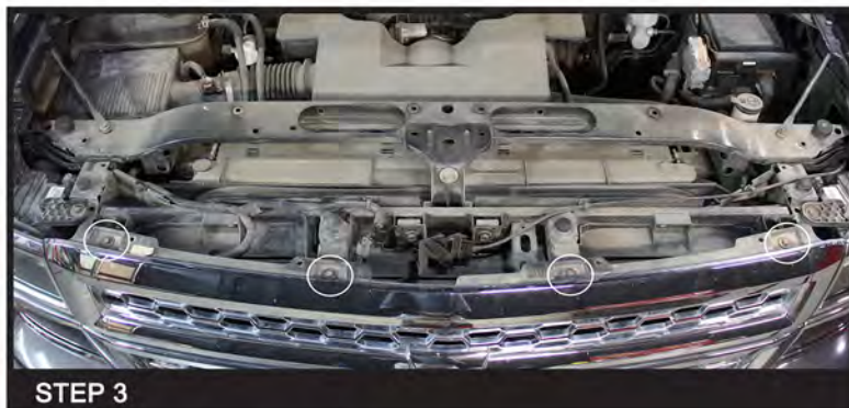
Remove the four 10mm upper grille mounting bolts
