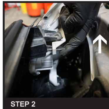
Loosen the top part of the front grille
