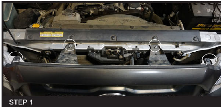
Remove the two plastic retainers and the two 10mm bolts
