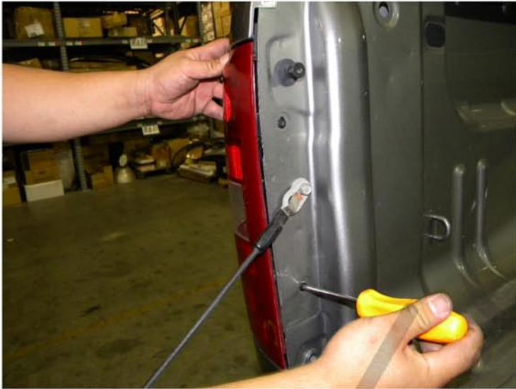
1. Remove the (2) Phillips head screws
