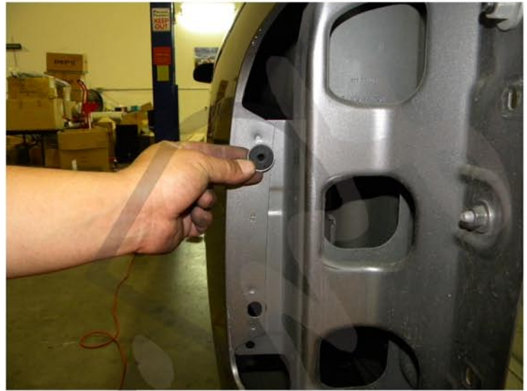
6. Replace the plastic holder onto the mounting holes
