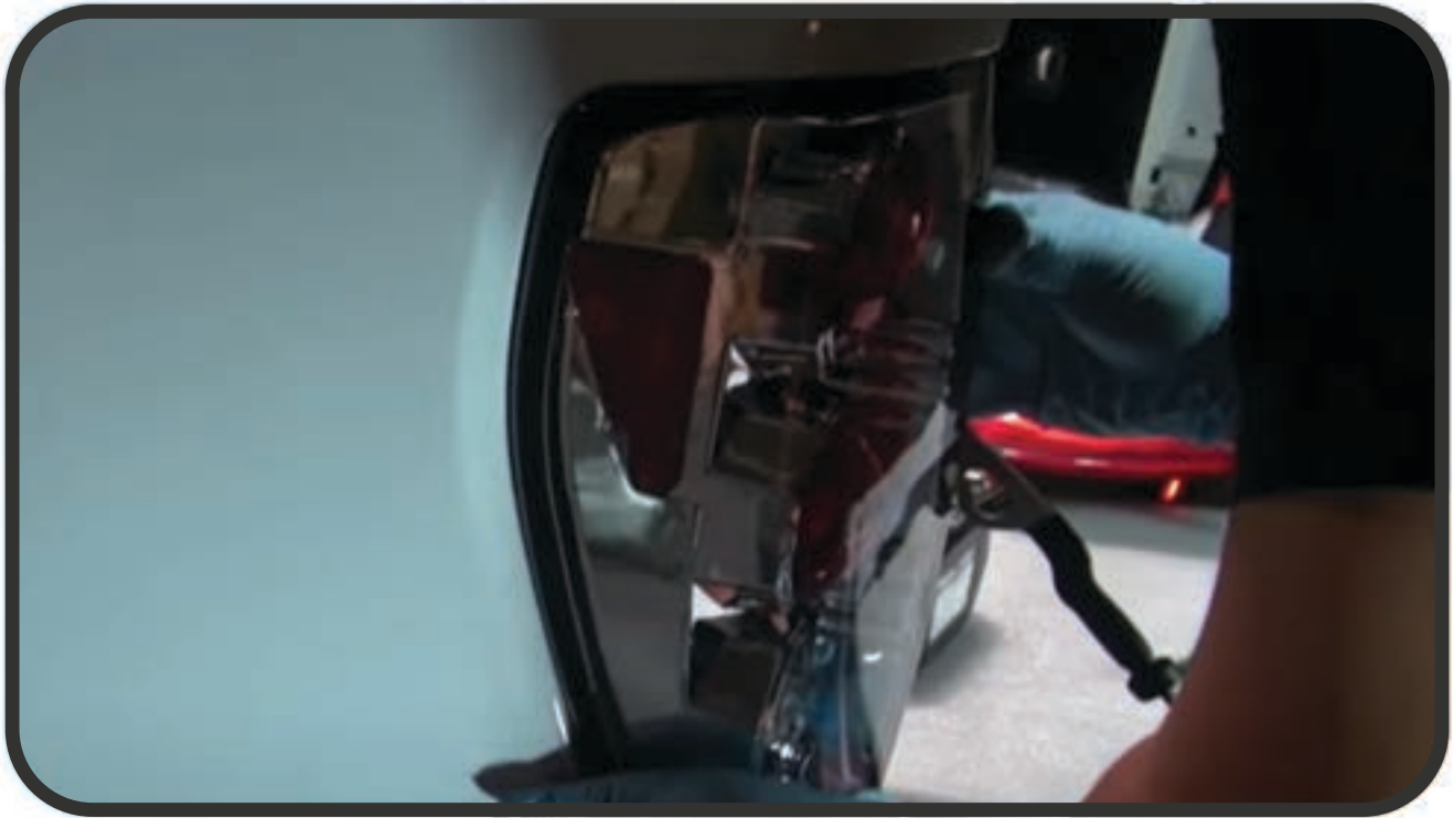
STEP 6: SEAT SPYDER TAIL LIGHT MAKING SURE NOT TO PINCH THE HARNESS
