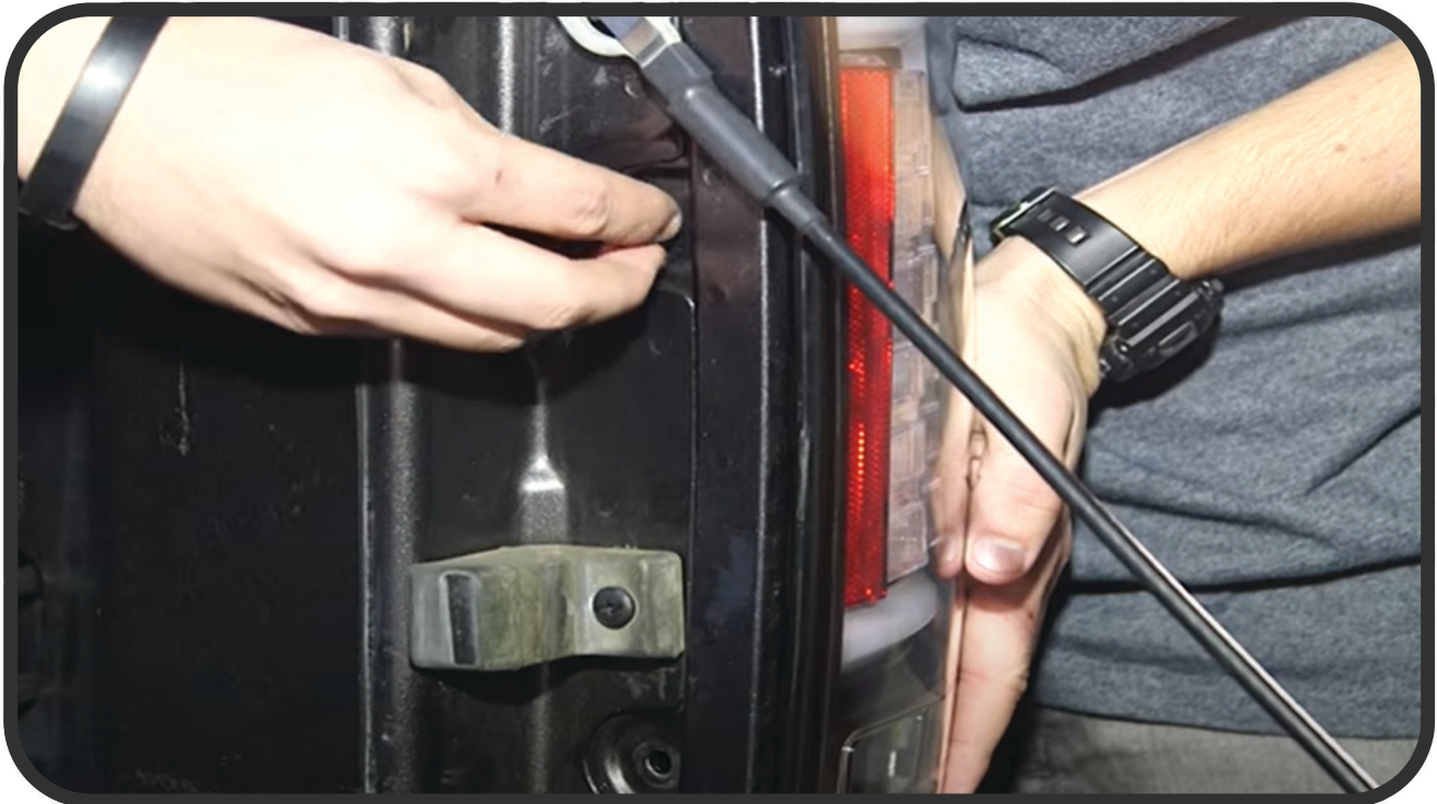
STEP 9: REINSTALL THE (2) T25 TORX SCREWS AND CLOSE THE TAILGATE
