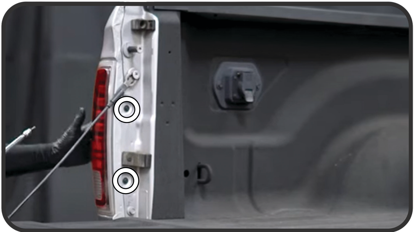
STEP 2: OPEN THE TAILGATE AND REMOVE (2) T20 TORX SCREWS
