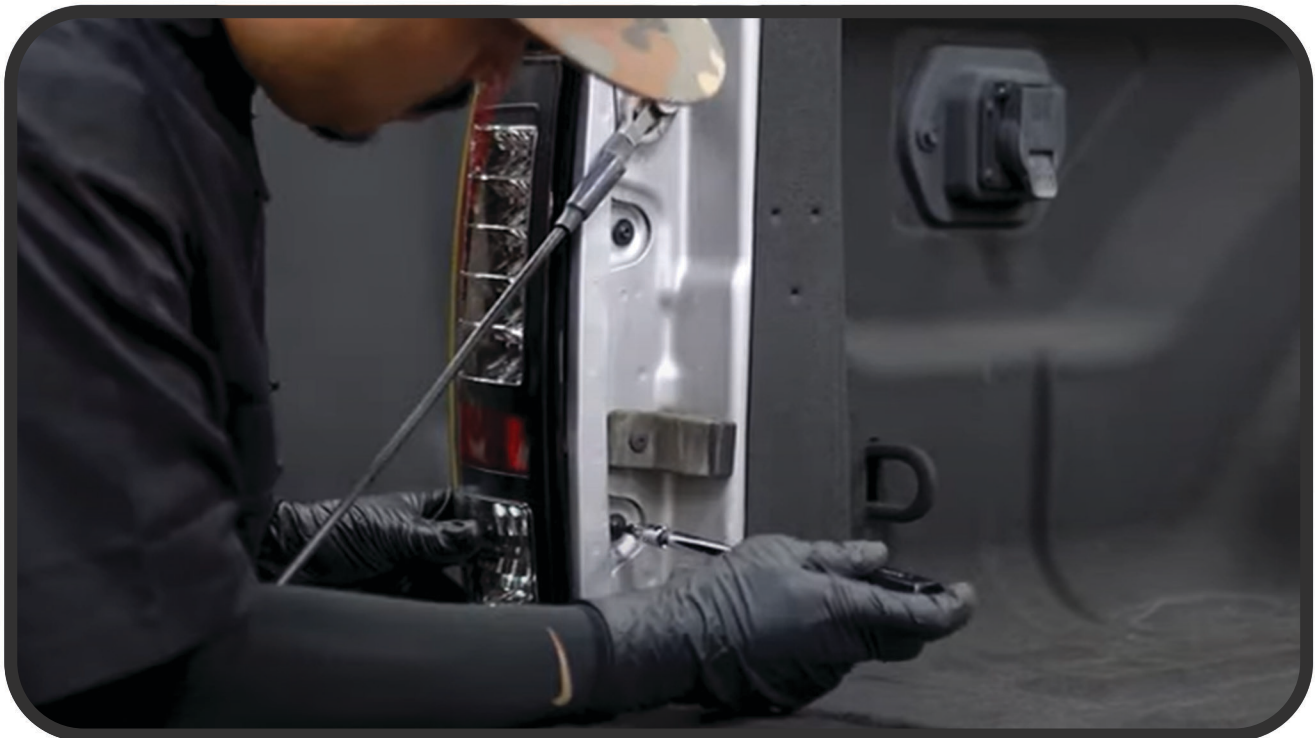
STEP 7: REINSTALL THE (2) T20 TORX SCREWS TO SECURE THE TAIL LIGHT. CLOSE THE TAILGATE
