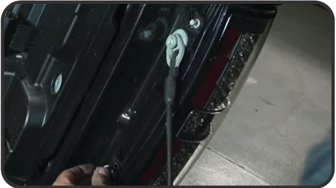
STEP 7: REINSTALL (2) 8MM BOLTS TO SECURE THE TAIL LIGHT
