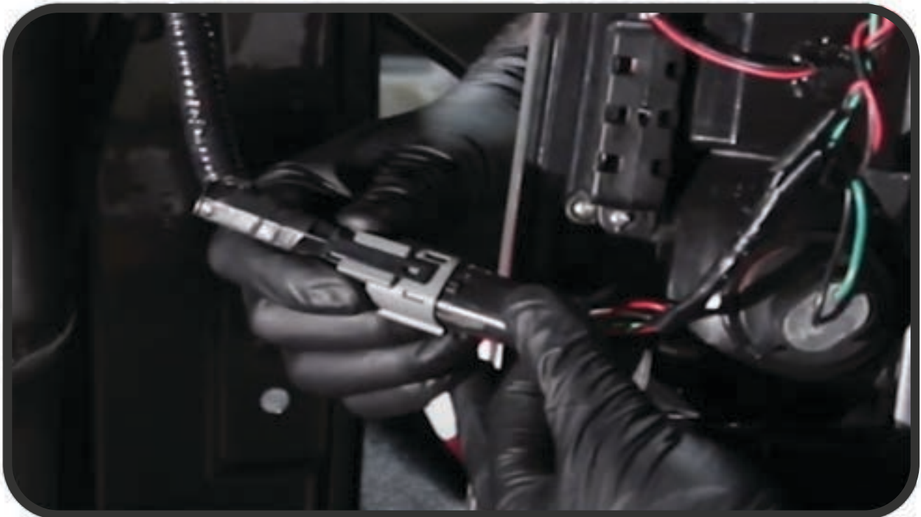
STEP 5: CONNECT SPYDER LED TAIL LIGHT HARNESS
