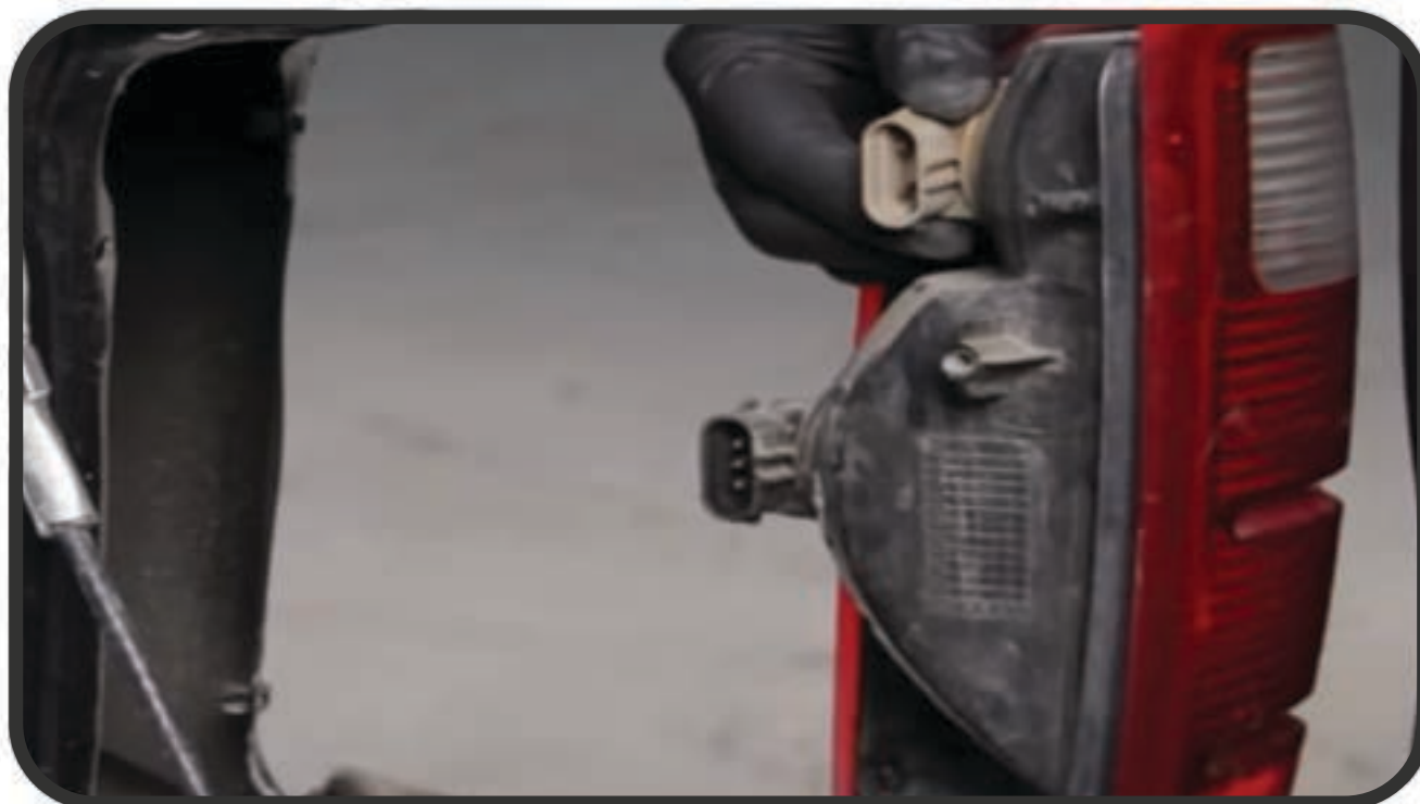
STEP 5: DISCONNECT BRAKE AND REVERSE LIGHT HARNESS
