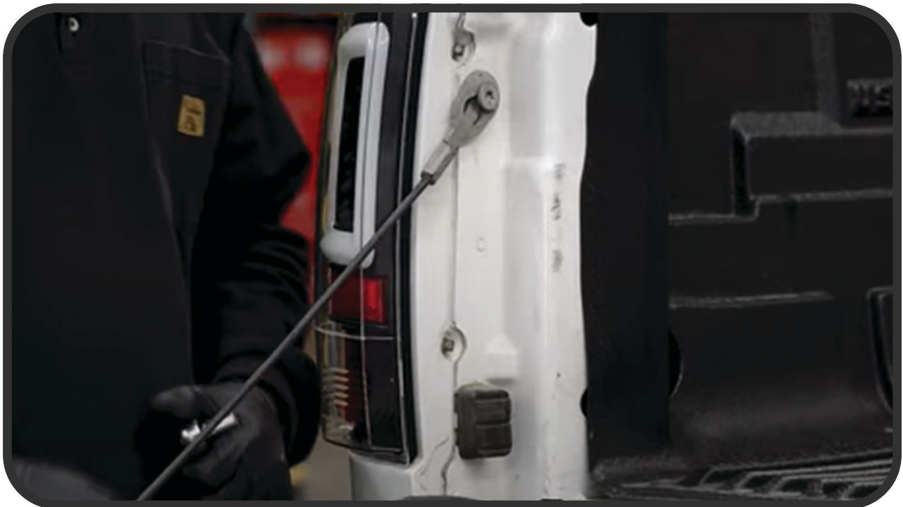
STEP 9: REINSTALL THE (2) 8MM BOLTS TO SECURE THE TAIL LIGHT
