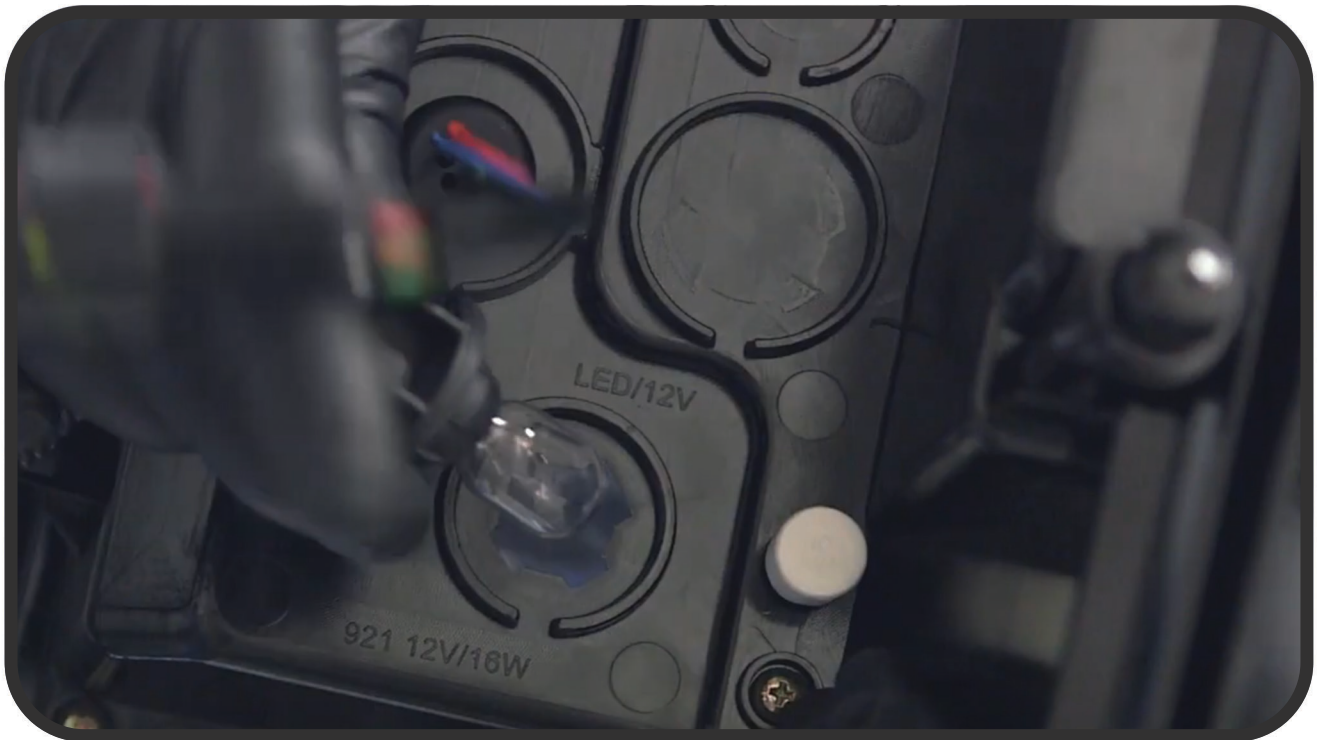
STEP 6: INSTALL REVERSE LIGHT SOCKET TO THE SPYDER TAIL LIGHT
