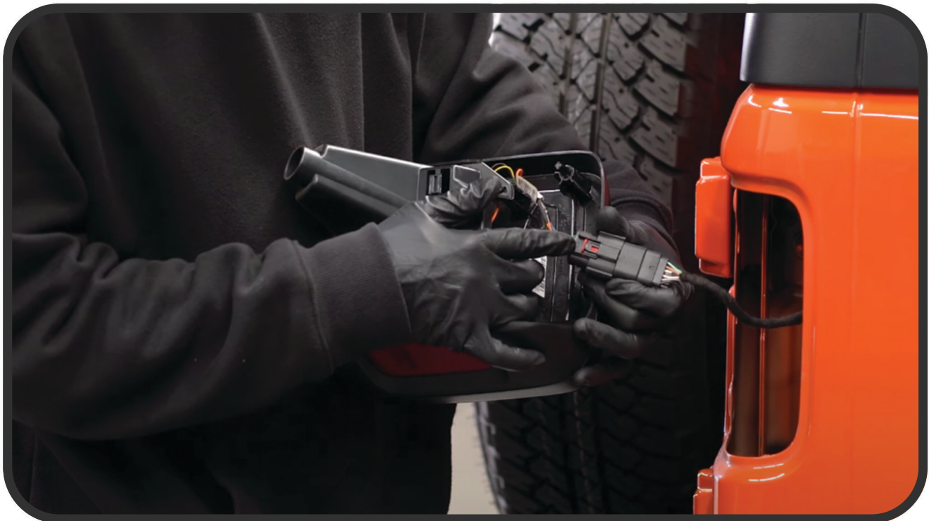
STEP 5: DISCONNECT THE TAIL LIGHT HARNESS BY PUSHING UP ON THE RED TAB TO UNLOCK IT
