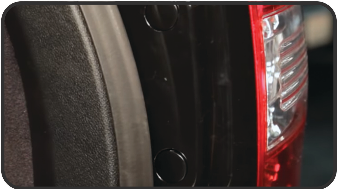
STEP 11: REMOVE THE (2) INCLUDED PLASTIC CAPS
