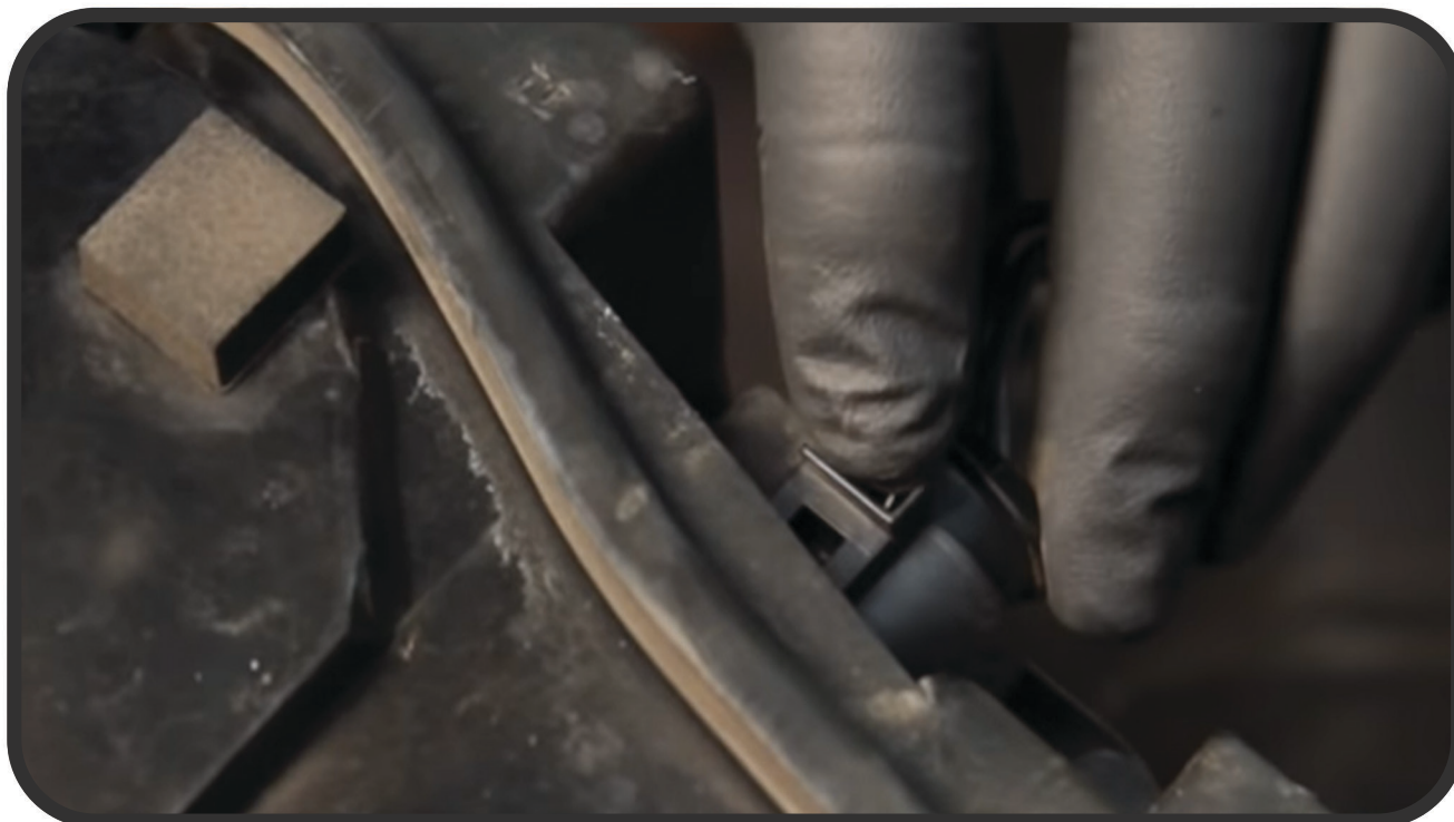
STEP 5: DISCONNECT THE TAIL LIGHT HARNESS
