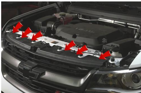
19. Reinstall (6x) T15 screws securing grill.
