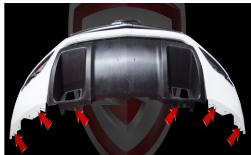
20. Reinstall (6x) 8mm bolts securing bottom of bumper fascia.
