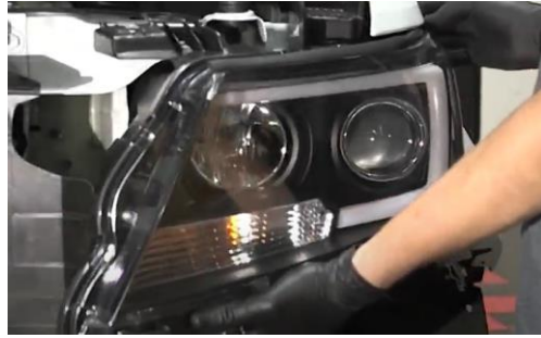
12. Disconnect headlight and turn signal harness.
