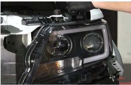
13. Reinstall (4x) 7mm bolts securing the headlight
