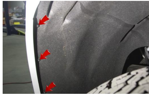
18. Install (3x) T15 torx screws securing fender liner.
