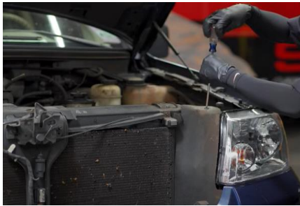
1. Remove (1x) phillips crew retainer.
