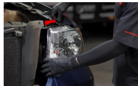
4. Carefully lift up on top bracket and unseat the headlight.
