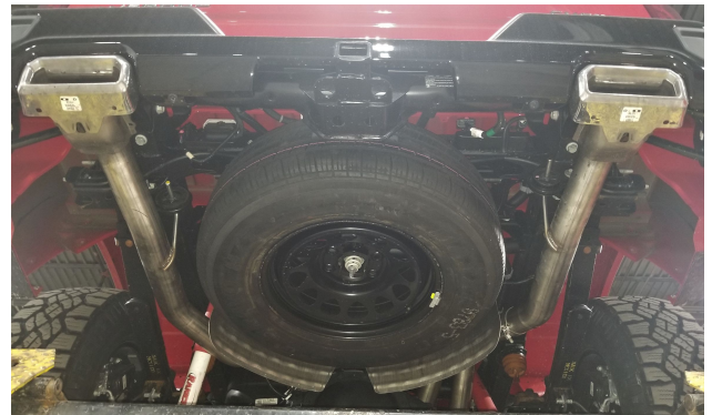
Detail 13: Rear tails and hanger brackets installed.
