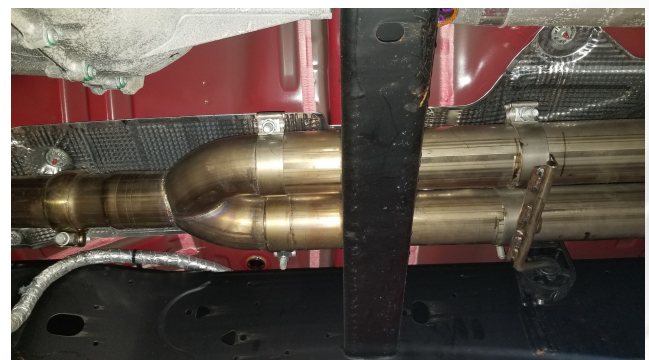
Detail 9: Y-pipe connection and inlet pipe hanger installed.
