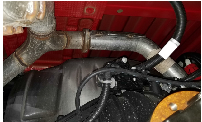
Detail 4: Left tail OEM flange connection
