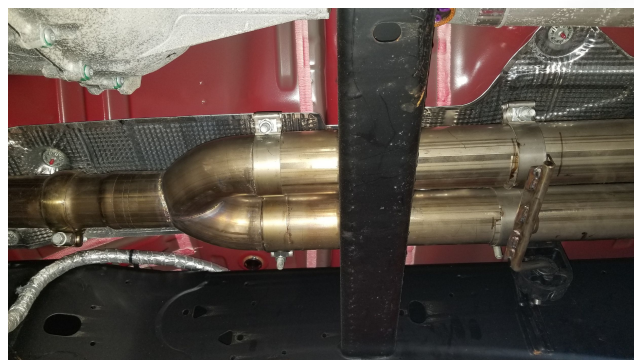
Detail 9: Y-pipe connection and inlet pipe hanger installed.
