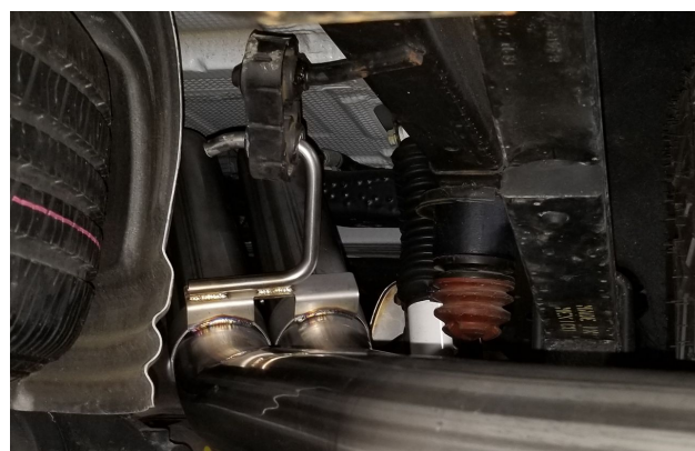
Detail 13: Rear tail hanger assembly, viewed from rear of vehicle.
