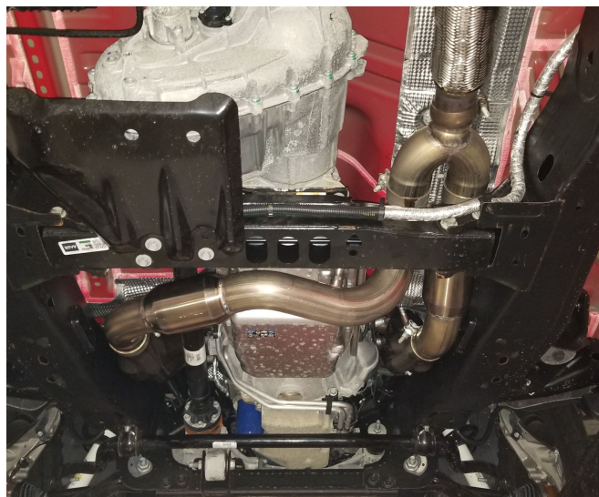
Detail 16: Headers and leads installed
