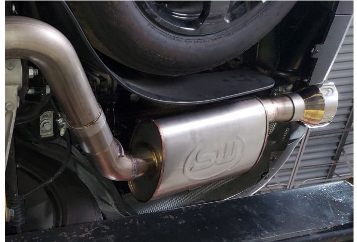
Detail 12: Right muffler assembly with tip installed
