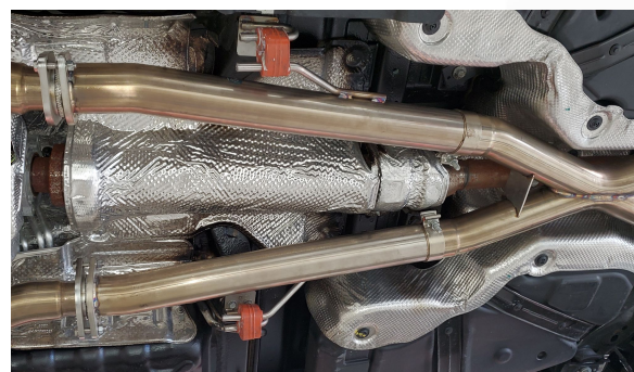
Detail 9: Inlets to X-pipe w/ hangers installed (Redline & SW headers shown)
