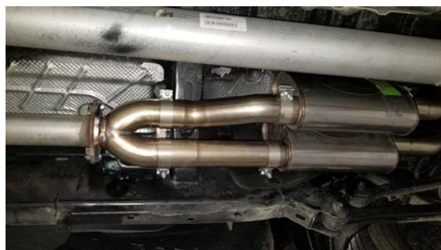
Detail 7: Factory Y-pipe connection shown
