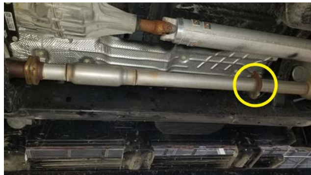
Detail 3: Rear OEM flange connection
