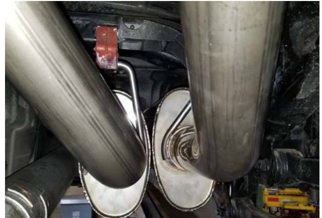
Detail 12: Orientation of hanger assemblies behind mufflers.
