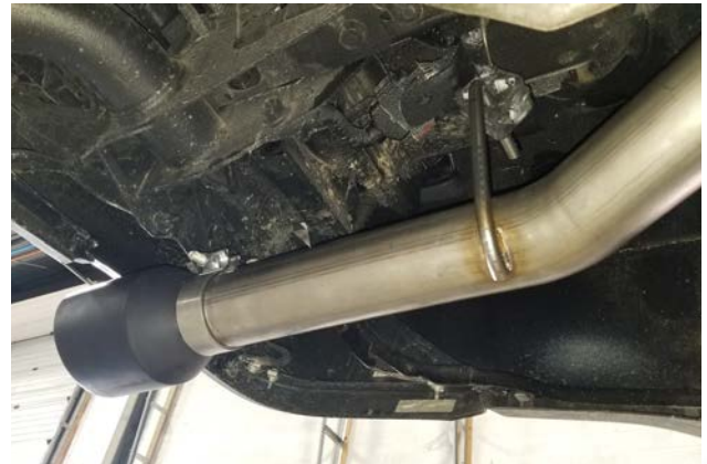
Detail 12: Rear tail section and tip installed.
