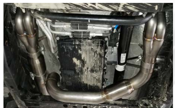
Detail 29: Headers and catted leads installed
