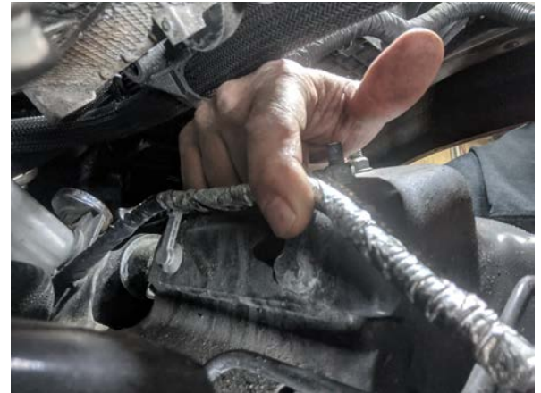
Detail 20a: Wire looms to be removed
