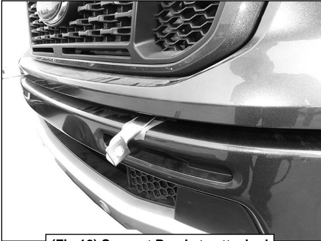
(Fig 12) Support Brackets attached
