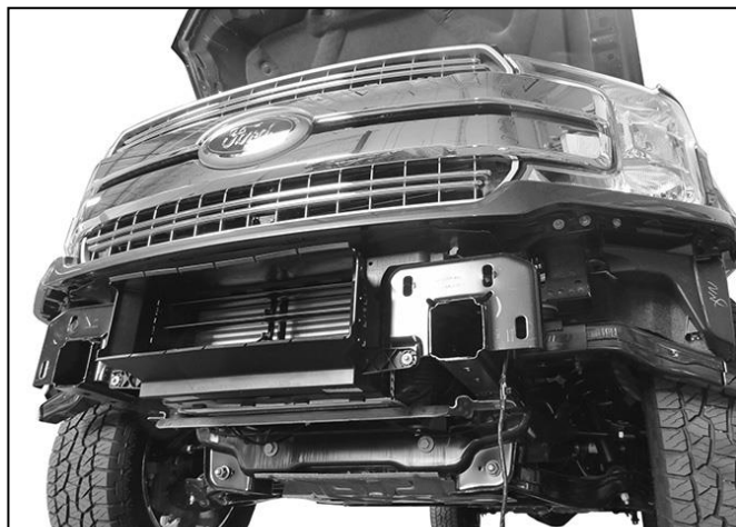
(Fig 18) 2018 models: Remove bumper assembly
